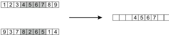
**Fig. 4.15.** Order crossover, step 1: copy randomly selected segment from first parent into offspring
